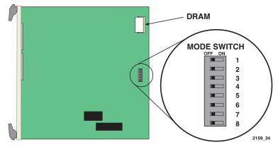
Figure B-1 Module Mode Switch Location/Component Layout
